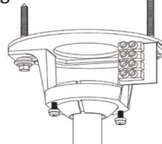
Place fan into hanger bracket and align Ball Joint Slot with hanger bracket as illustrated. (See Fg.3)
