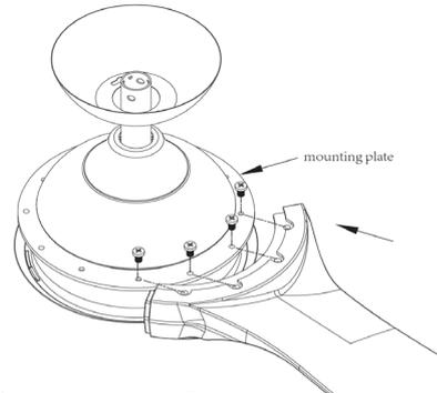
Attach the blade to the top of the motor using the 4 blade screws provided. Tighten the screws and repeat this procedure for all blades. (See Fig. 6)
