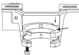
Secure the hanger bracket to ceiling beam or a suitable piece of timber inserted between the ceiling beams using the two long screws supplied with the package. (See Fg.1)
