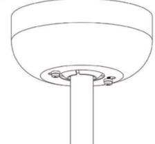
After wiring is completed, attach the canopy to the hanger bracket by pushing upwards and twisting anti-clockwise. Tighten screws and ensure canopy is not touching the ball joint. (See Fg.4)
