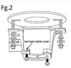
Place circular shockproof gasket above the hanger bracket. Align the bracket and screw the hanger bracket to the ceiling tightly. (See Fg.2)
